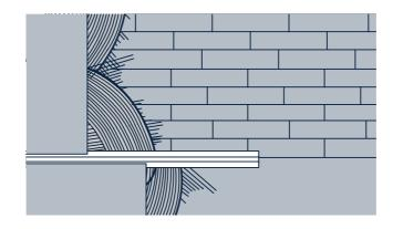
If there are joints between surfaces of different types (e.g. reinforced concrete and bricks), it is mandatory to install an expansion joint.
