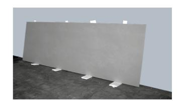
For upright storage, place the long side of the slab on wooden planks.
