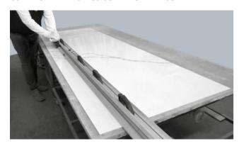
A practical tool for cutting is the tile cutter ruler (for instance Keracut by Sigma or Raizor by Raimondi). For 3plus, 5plus and 6plus Kerlite, after scoring the ceramic surface with this tool and splitting the slab, complete the operation by cutting the fibreglass mesh with a standard cutter. It is recommended to use this tool to cut polished surfaces, exerting strong pressure on the carriage mounted on the guide.
