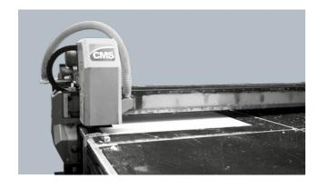
Kerlite can be cut by scoring. This operation must be performed on a cutting bench and on the front face of the slab.
