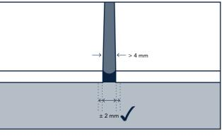
A test is conducted on the floor and wall tiling. This test consists in an initial evaluation of the appearance of the slabs, in order to verify the presence of any disturbing effects due to visual differences in the width of the grout.
