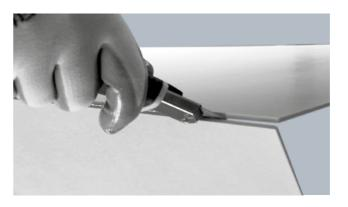
For 3plus, 5plus and 6plus Kerlite, after scoring the ceramic part and splitting the slab, complete the operation by cutting the fibreglass mesh with a standard cutter.
