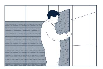
Laying of a protective cardboard on the installed wall
