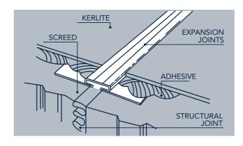
In line with a structural joint in the screed, it is mandatory to install an expansion joint with a width that is at least the size of the existing one
