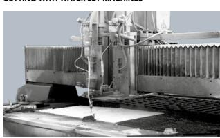
Kerlite can be cut with water jet cutting machines. The feed rate of this operation should be between 2 and 3 m/min.
