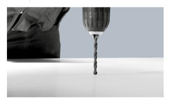
As far as manual drilling is concerned, use tungsten bits with a diameter up to 10 mm, fitted to electric drills or battery-operated screwdrivers.
