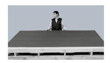
100x300 cm and 120x260 cm slabs of Kerlite can be lifted by one person. Lift the slab with open hands. Slowly raise the longer side so as to eliminate the suction effect, due to contact with the underlying slab, and ensure a good grip. When handling the use of gloves is recommended.
