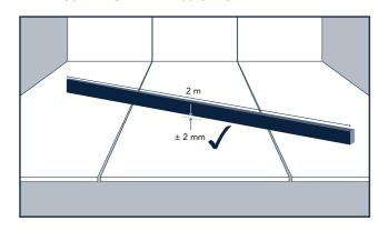
Flatness must be measured on the floor and wall tiling. It is checked by using a levelling rod with a length of at least 2 metres. Place the rod on the substrate in all directions.
