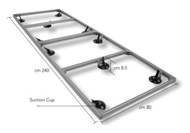
To safely handle and install 100x300 cm and 120x260 cm Kerlite slabs, a special frame is available upon request. It is made of aluminium and features suction cups. It is ideal for installing on scaffolding at a height of over 2 metres.
